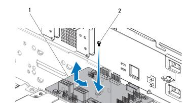
Figure 3-25. Removing and Installing the Fan Controller Board
